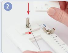
Remove the plate and place the looped wire/cord around the post. Replace the plate.
